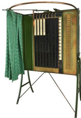
The advantages of gear-and-lever voting machine, c. 1898, over the ballot box were many, including that it kept a running count, thus speeding up the reporting of results. (Hugh Talman, NMAH)
